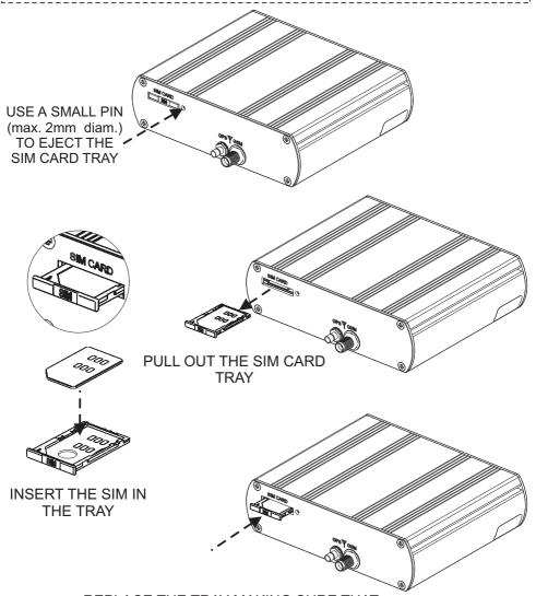
REPLACE THE TRAY MAKING SURE THAT THE "SIM" LABEL ON THE TRAY IS ALIGNED WITH THE SIM CARD MARKING ON THE UNIT.
